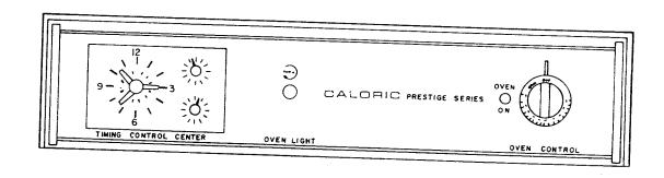
Some models have an electric clock with a minute timer and an automatic "START" and "STOP" timing system. The clocktimer is located on the left side of the control panel. The clock conveniently gives you the time of day as well as a 60 minute timer. The knob on the clock face is used to set the time. Push in and turn the knob clockwise to the correct time.
